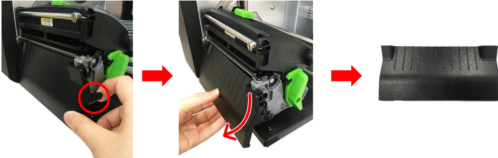
4. Reverse the steps to install the lower front panel.
