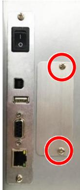
4. Connect the two slot-in Wi-Fi & Bluetooth module cables on the main board.
