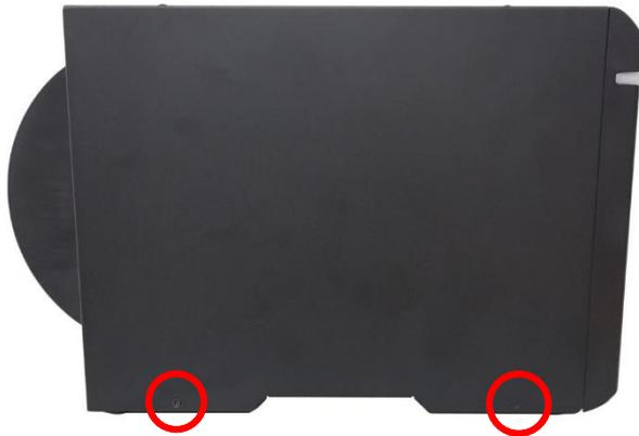
4. Lift up and pull as indicated to remove the electronics cover from the printer.
