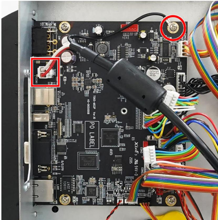
4. Remove the three screws securing the power supply unit in place.
